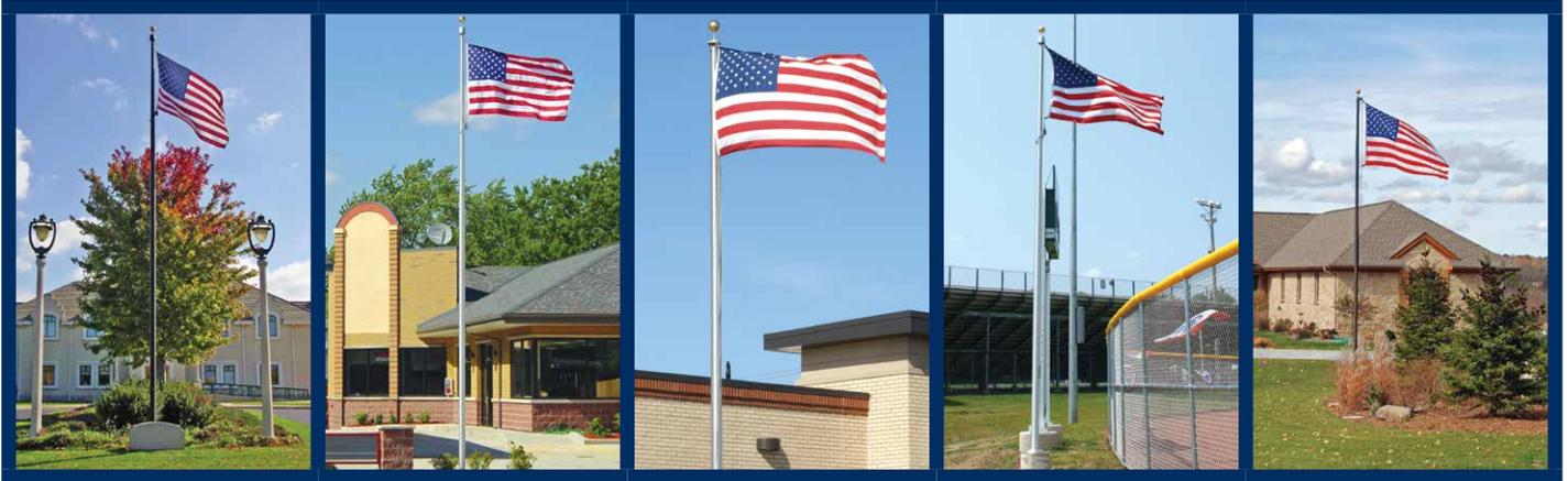
Our cone tapered ground set aluminum flagpoles are precision fabricated from new, 6063-T6 tubing utilizing the industry's most sophisticated manufacturing processes. The conical portion tapers approximately 1" in every 5-1/2 feet.
